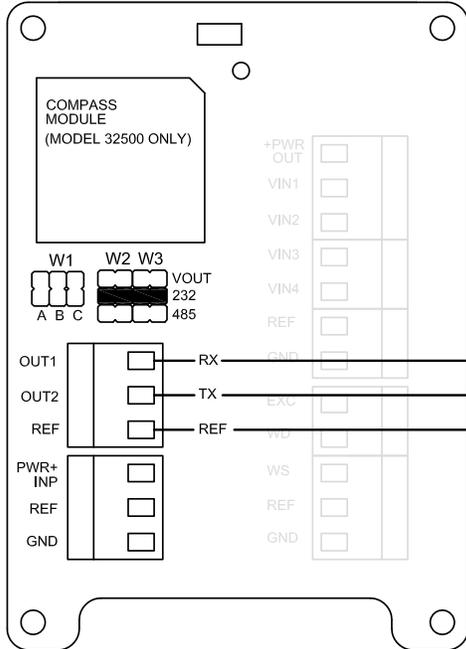
Typical RS-232 connection to PC or other device. 32400/500 jumpers set for RS-232 ASCII output.
