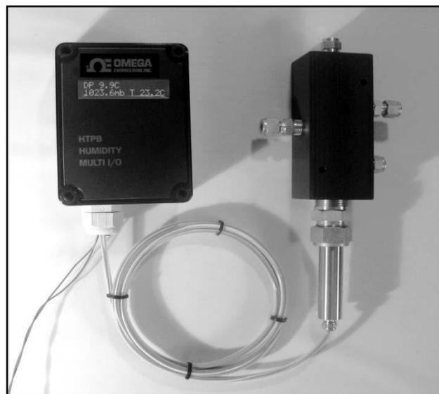
Figure 3-1, System with Sample Cell, ready for mounting
